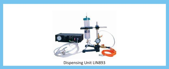
The unit LIN 893 is a semi-automatic paste dispensing machine. The dispenser use the low-pressure air within time to set for, use the pedal control to put out the paste. Very flexible adjustment is manual
